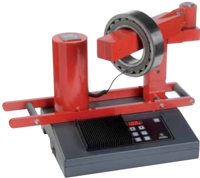
BETEX 24 RSD TURBO, 3.6 kVA Bench-top type with swivel arm for ergonomic operation. Heats parts in horizontal or vertical position. Choice of 5 yokes. Min. Ø 15 mm. Max. outside diameter 520 mm. (With extension yokes 750 mm). Suitable for bearings up to ± 95 kg.
